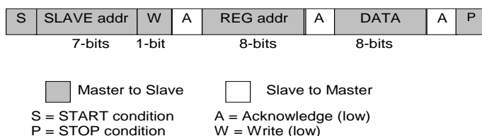
Figure 27: I 2 C byte write (SDA signal)
