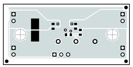
Figure 3. Bottom Layer Routing
