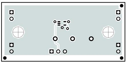
Figure 2. Top Layer Routing
