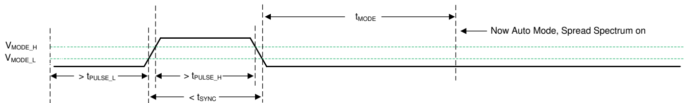
Figure 8-10. Transition from SYNC Mode to Auto Mode
