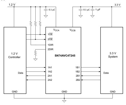
Figure 5. Typical Application Diagram
