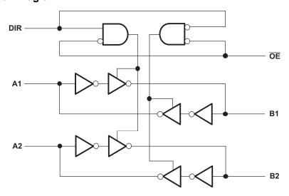
Figure 4. Logic Diagram (Positive Logic) for 1/2 of SN74AVC4T245
