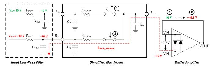
Figure 7-2. Back-to-Back Diodes Create Settling Issues
