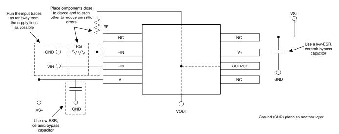
Figure 8-4. Operational Amplifier Board Layout for Noninverting Configuration
