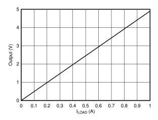
Figure 8-2. Low-Side, Current-Sense, Transfer Function
