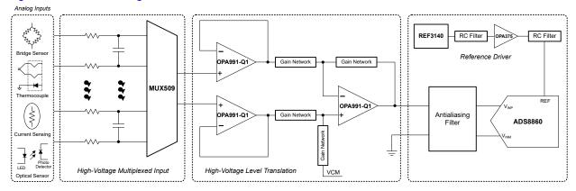
OPAx991-Q1 in a High-Voltage Signal Chain
