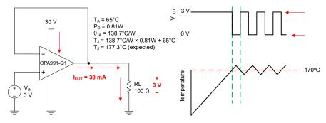
Figure 7-4. Thermal Protection
