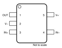
Figure 5-1. OPA991-Q1 DBV Package, 5-Pin SOT-23 (Top View)
