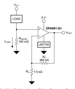
Figure 8-1. OPAx991-Q1 in a Low-Side, Current-Sensing Application
