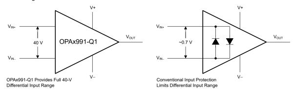
Figure 7-1. OPAx991-Q1 Input Protection Does Not Limit Differential Input Capability
