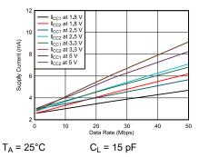
Figure 6-3. ISO6731-Q1 Supply Current vs Data Rate (With 15-pF Load)
