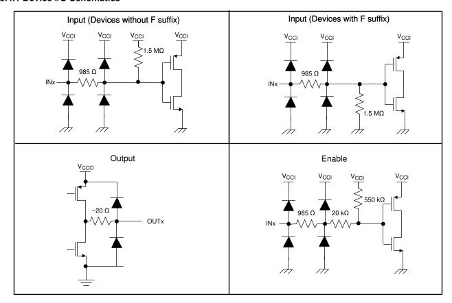
Figure 8-3. Device I/O Schematics
