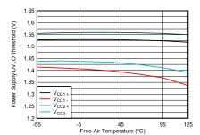
Figure 6-7. Power Supply Undervoltage Threshold vs Free-Air Temperature
