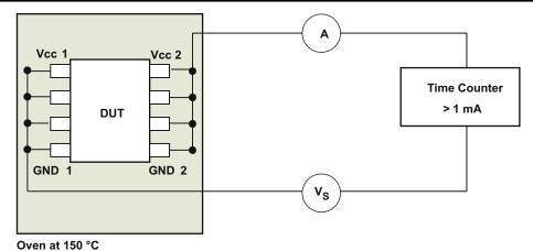
Figure 9-7. Test Setup for Insulation Lifetime Measurement
