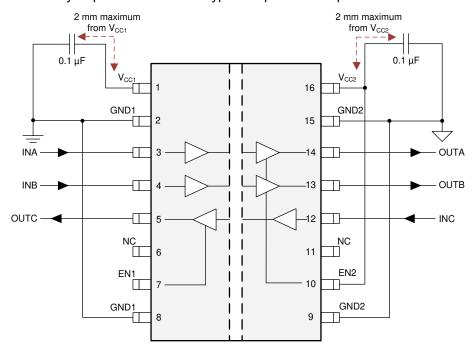
Figure 9-2. Typical ISO6731-Q1 Circuit Hook-up
