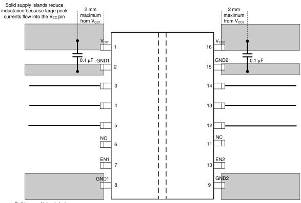
Solid ground islands help dissipate heat through PCB
