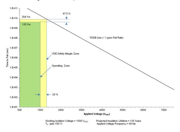
Figure 9-8. Insulation Lifetime Projection Data
