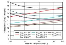
Figure 6-8. Propagation Delay Time vs Free-Air Temperature
