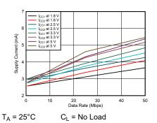
Figure 6-4. ISO6731-Q1 Supply Current vs Data Rate (With No Load)
