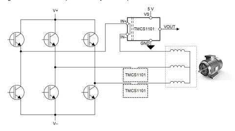
Figure 10-2. Inline Motor Phase Current Sensing
