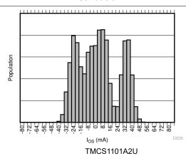
Figure 7-12. Input Offset Current Production
