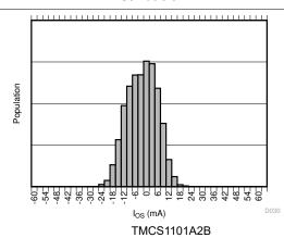
Figure 7-11. Input Offset Current Production Distribution
