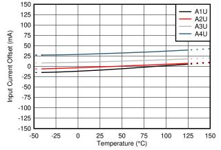
Figure 9-3. Offset Error Drift Across Temperature (U Variants)
