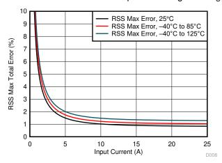
Figure 10-1. RSS Error vs. Input Current
