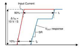
Figure 8-4. Current Overload Transient Response
