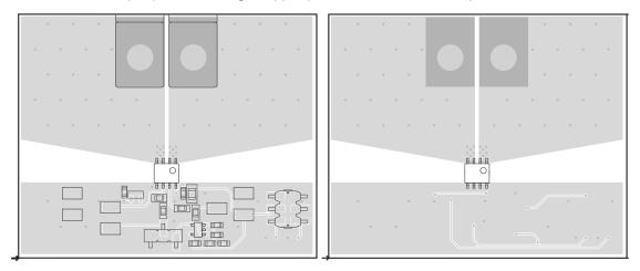
Figure 12-3. Recommended Board Top (Left) and Bottom (Right) Plane Layout
