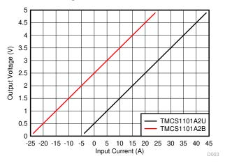
Figure 9-14. Output Voltage Relationship to Input Current for TMCS1101A2B and TMCS1101A2U
