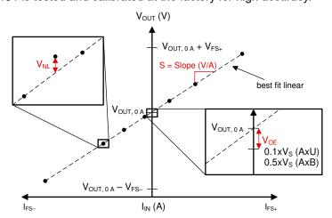
Figure 8-1. Sensitivity, Offset, and Nonlinearity Error
