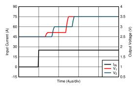
Figure 8-2. Transient Step Response
