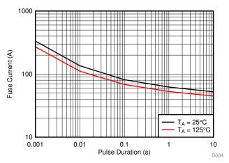
Figure 8-10. Single-Pulse Leadframe Capability
