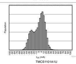
Figure 7-10. Input Offset Current Production
