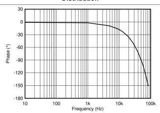
Figure 7-18. Phase vs. Frequency, All Gains
