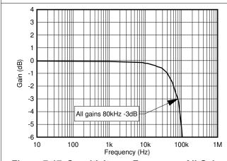
Figure 7-17. Sensitivity vs. Frequency, All Gains Normalized to 1 Hz
