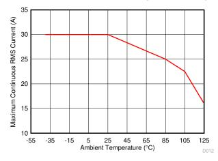
Figure 8-5. Maximum Continuous RMS Current vs. Ambient Temperature
