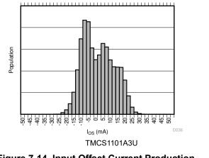
Figure 7-14. Input Offset Current Production Distribution
