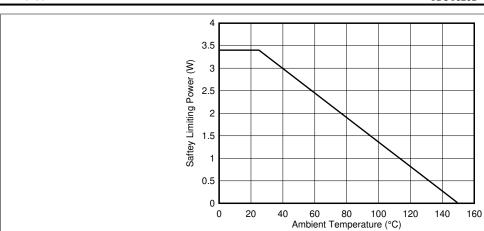
Figure 7-30. Thermal Derating Curve for Safety-Limiting Power
