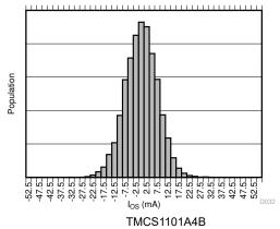
Figure 7-15. Input Offset Current Production
