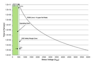
Figure 9-1. Insulation Lifetime
