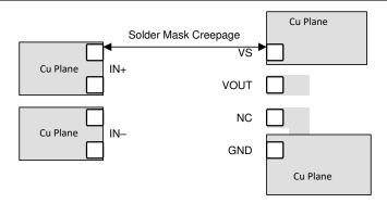
Figure 12-2. Layout for System Creepage Requirements
