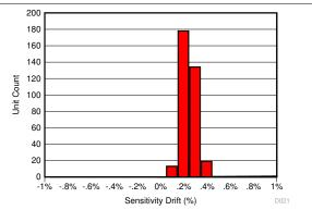
Figure 9-7. Sensitivity Error Drift After AEC-Q100 High Temperature Operating Life Stress Test
