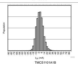
Figure 7-9. Input Offset Current Production Distribution
