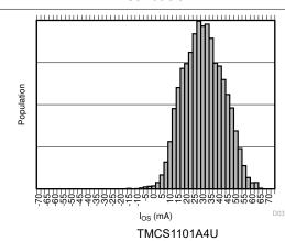
Figure 7-16. Input Offset Current Production
