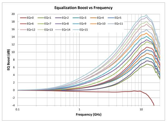
Figure 6-1. Typical EQ Boost vs Frequency
