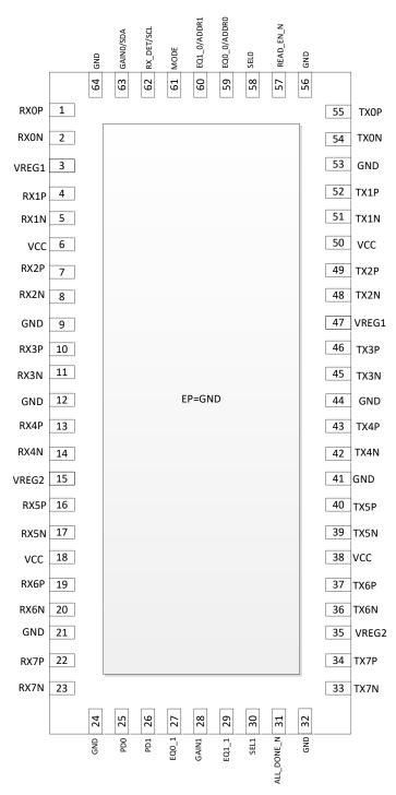
Figure 5-1. NJX Package 64-Pin WQFN Top View
