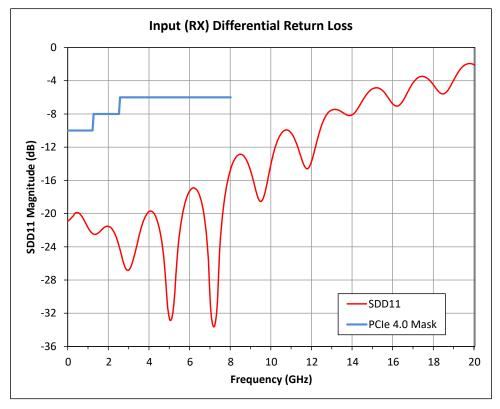
Figure 6-3. Typical RX Differential Return Loss
