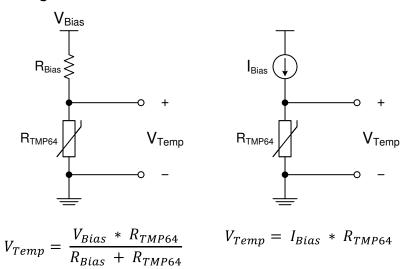
Figure 8-1. Typical Implementation Circuits
