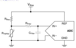
Figure 9-2. TMP64 Voltage Divider With an ADC
