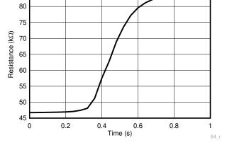
TMP64: Stirred Liquid. Temperature: 25 °C to 125 °C
