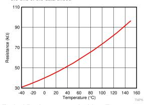
**Typical Resistances vs Ambient Temperature**
