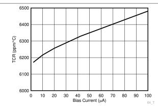
Figure 7-3. TCR as a Function of Sense Current,  $\rm I_{SNS}$
