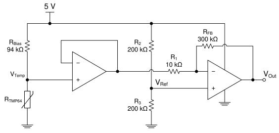
Figure 9-6. Thermal Foldback Using TMP64 Voltage Divider and a Rail-to-Rail Op Amp
