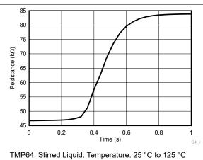
Figure 7-8. DEC Thermal Response Time
