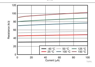
Figure 7-5. Supply Dependence Resistance vs.
