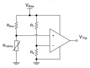
Figure 9-5. Temperature Switch Using TMP64 Voltage Divider and a Comparator
