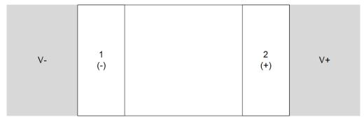
Figure 11-1. Recommended Layout: DEC Package
