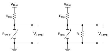
Figure 9-4. TMP64 vs. NTC With Linearization Resistor (R<sub>P</sub>) Voltage Divider Circuits
