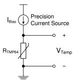
Figure 9-3. TMP64 Biasing Circuit With Current Source
