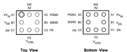
Figure 3. 8-Bump Thin DSBGA Package, Large Bump
