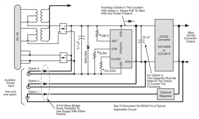
Figure 21. Auxiliary Power ORing
