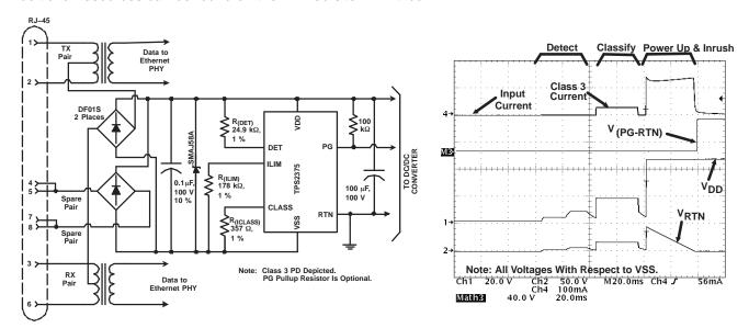
Figure 1. Typical Application Circuit and Startup Waveforms
