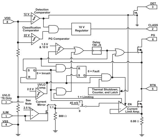
Note: For the TPS2376, the UVLO comparator connects to the UVLO pin and not to the UVLO divider.
