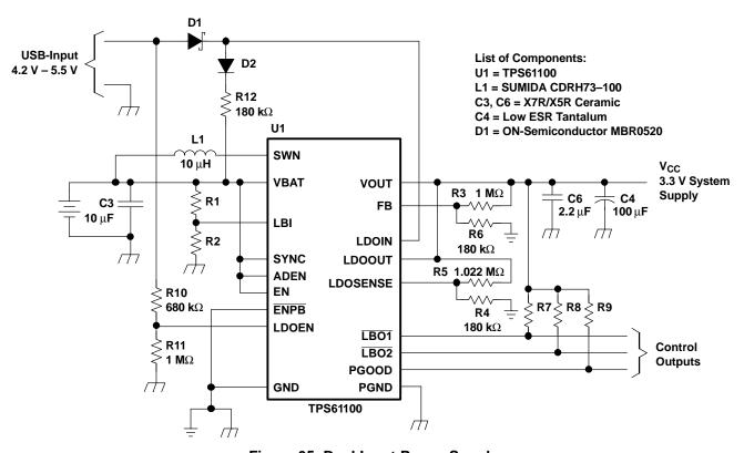
Figure 35. Dual Input Power Supply
