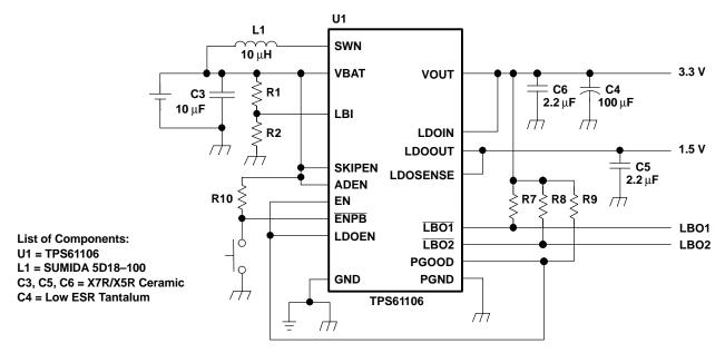
Figure 34. Simple Solution Using a Pushbutton for Start-Up
