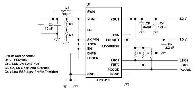
Figure 30. Low Profile Solution, Maximum Height 1,8 mm
