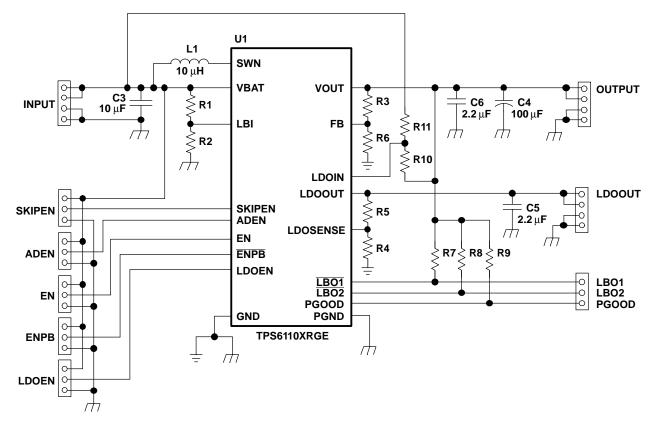
Figure 36. TPS6110x EVM Circuit Diagram
