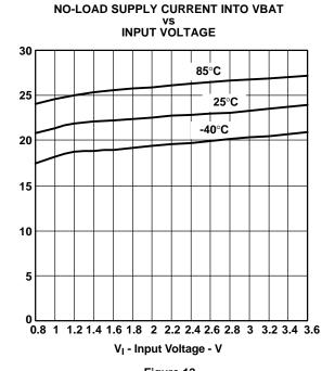
No-Load Supply Current Into VBAT -  $\,\mu\text{A}$
