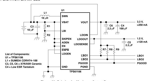
Figure 29. Solution for Maximum Output Power
