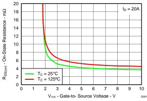
Figure 7. On Resistance vs. Gate Voltage
