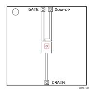
Max  $R_{\theta JA} = 123^{\circ}C/W$  when mounted on minimum pad area of 2 oz. Cu.
