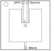
Max  $R_{\theta JA} = 50^{\circ} C/W$  when mounted on 1 inch<sup>2</sup> of 2 oz. Cu.
