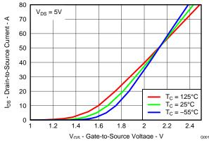
Figure 3. Transfer Characteristics
