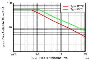
Figure 11. Single Pulse Unclamped Inductive Switching
