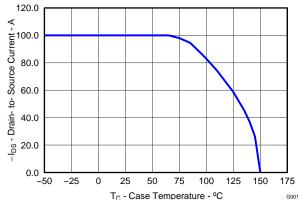
Figure 12. Maximum Drain Current vs. Temperature
