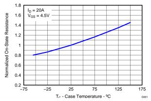
Figure 8. Normalized On Resistance vs. Temperature
