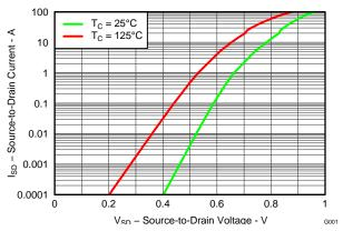
Figure 9. Typical Diode Forward Voltage
