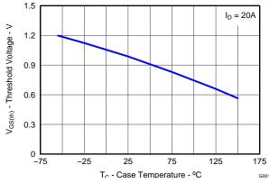
Figure 6. Threshold Voltage vs. Temperature
