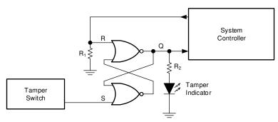
Figure 9-1. Typical Application Block Diagram
