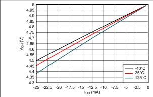
Figure 6-1. Output Voltage vs Current in HIGH State; 5-V Supply
