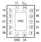
Figure 5-2. SN74AHCT02 RGY or BQA Package, 14-Pin (Top View)
