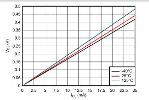
Figure 6-2. Output Voltage vs Current in LOW State; 5-V Supply
