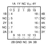
Figure 5-3. SN54AHCT02 FK Package, 20-Pin (Top View)
