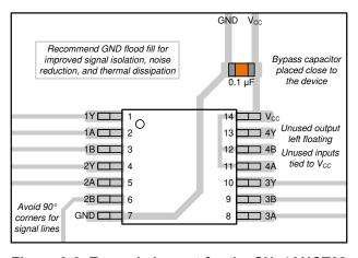
Figure 9-3. Example Layout for the SNx4AHCT02
