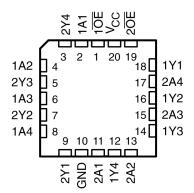
Figure 4-2. SN54AC244 FK Package (Top View)
