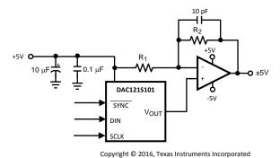
Figure 33. Bipolar Operation
