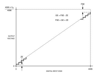
Figure 1. Input / Output Transfer Characteristic
