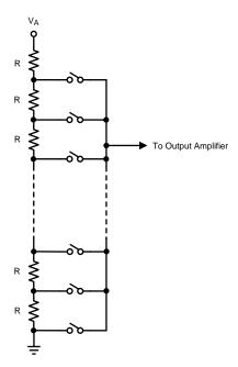
Figure 30. DAC Resistor String
