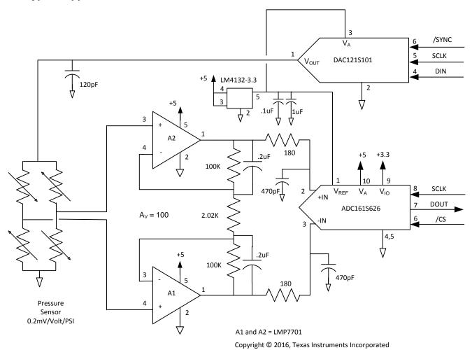
Figure 38. Pressure Sensor Gain Adjust
