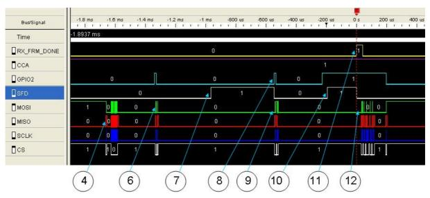
Figure 15 Capture of packet transmission scenario using a logic analyzer
