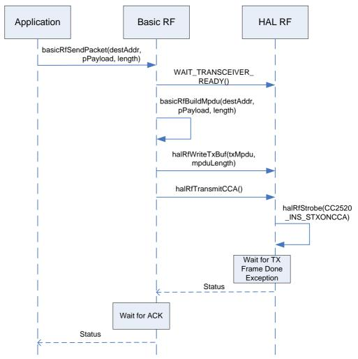
Figure 14 Packet transmission
