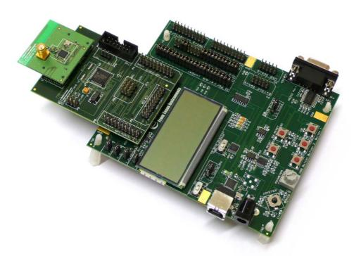
Figure 1 SmartRF05EB/CCMSP2618/CC2520EM
