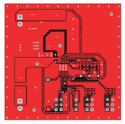
Figure 6. Top Layer Routing
