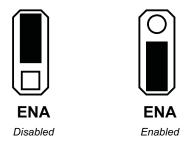
Figure 2. Enable Jumper Settings
