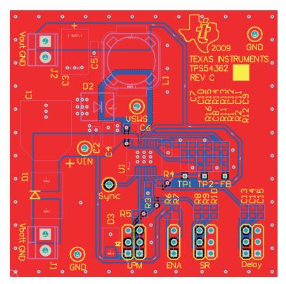
Figure 5. Top Assembly Layer
