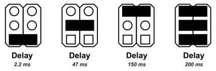
Figure 4. Reset Delay Time Settings
