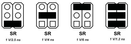
Figure 3. Slew Rate Settings
