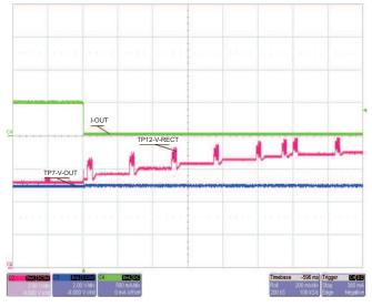
Figure 4. Load Dump, 500mA to 0mA
