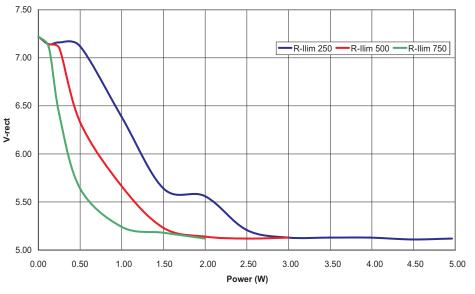
Figure 9. bq51013AEVM-764 V-rect vs Output Power
