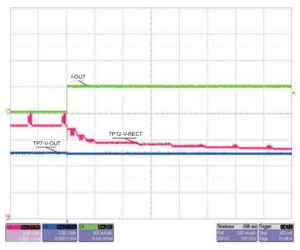
Figure 3. Load Step, 0mA to 500mA
