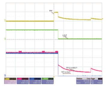
Figure 7. Equipment Shutdown Wireless Disable
