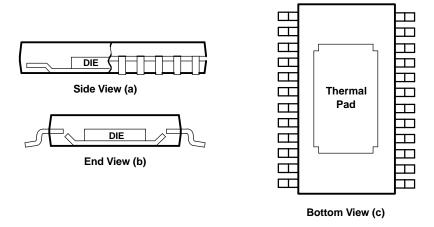
Figure 41. Views of Thermally Enhanced PWP Package
