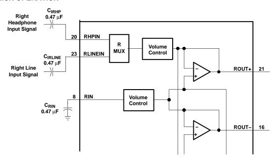
Figure 48. TPA0112 Example Input MUX Circuit
