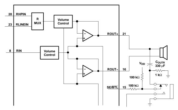
Figure 47. TPA0112 Resistor Divider Network Circuit
