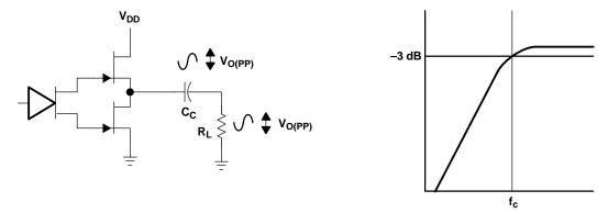
Figure 45. Single-Ended Configuration and Frequency Response
