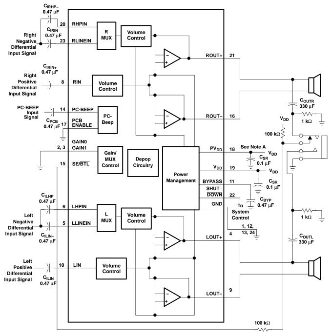
A. A 0.1-μF ceramic capacitor should be placed as close as possible to the IC. For filtering lower frequency noise signals, a larger electrolytic capacitor of 10 μF or greater should be placed near the audio power amplifier.
