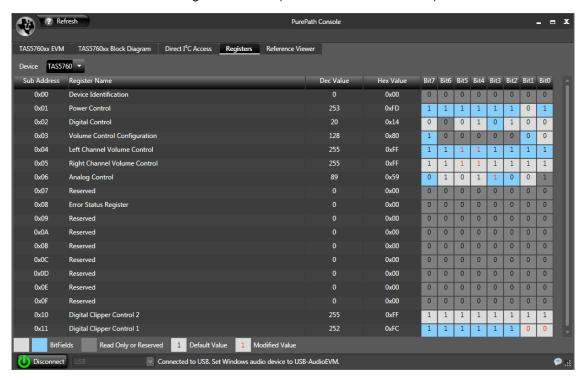
Figure 11. Device Registers Tab
