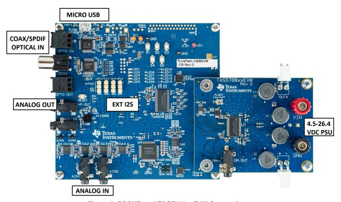
Figure 3. PPCMB and TAS5760xxEVM Connection
