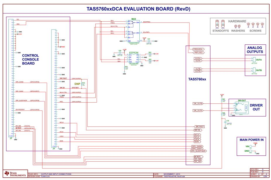
Figure 15. TAS5760xxEVM Rev D Schematic (Page 2 of 2)
