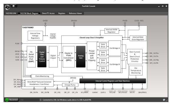
Figure 7. TAS5760 Block Diagram
