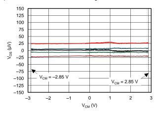
Figure 41. Offset Voltage vs Common-Mode Voltage (Zero-Crossover)
