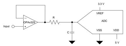
Figure 45. The OPA2325 as an Input Driver for ADCs
