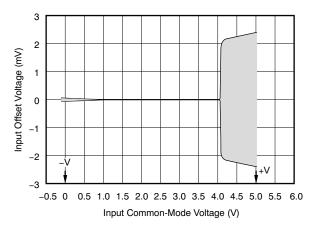
Figure 40. Input Common-Mode Voltage vs Input Offset Voltage (Traditional Rail-to-Rail Input CMOS Amplifiers)
