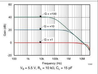
Figure 24. Closed-Loop Gain vs Frequency
