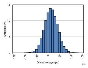
Figure 42. Offset Voltage Distribution
