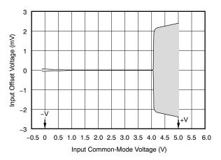
Figure 48. Input Offset Voltage vs Common-Mode Voltage (For Traditional Rail-to-Rail Input CMOS Amplifiers)
