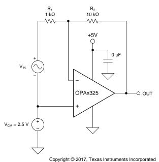
Figure 44. Basic Single-Supply Connection
