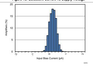
Figure 12. Input Bias Current Distribution Histogram
