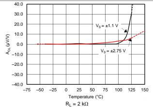
Figure 7. Open-Loop Gain vs Temperature
