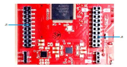
Figure 5. 20-Pin Obstacle Detection Sensor Connectors
