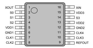
Package: 16-Pin SSOP(Top View)
