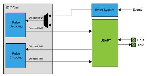
The USART is set in IRCOM mode by writing  $0 \times 0.2$  to the CMODE bit field in the USARTn.CTRLC register. The data on the TXD/RXD pins are the inverted values of the transmitted/received infrared pulse. It is also possible to select an event channel from the Event System as an input for the IRCOM receiver. This enables the IRCOM to receive input from the I/O pins or sources other than the corresponding RXD pin, which will disable the RxD input from the USART pin.
