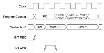
If an interrupt occurs during the execution of a multi-cycle instruction, the instruction is completed before the interrupt is served, as shown in the following figure.
