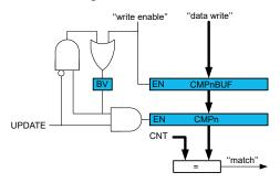
Both the TCAn.CMPn and TCAn.CMPnBUF registers are available as I/O registers, allowing the initialization and bypassing of the buffer register and the double-buffering function.
