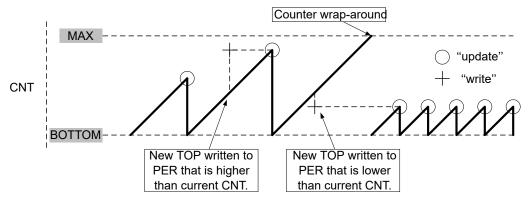
A counter wrap-around can occur in any mode of operation when counting up without buffering, as the TCAn.CNT and TCAn.PER registers are continuously compared. If writing a new TOP value to TCAn.PER lower than the current TCAn.CNT, the counter will wrap first before a compare match occurs.
