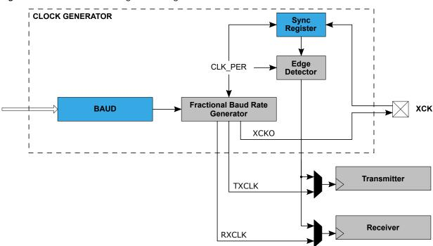
Figure 25-3. Clock Generation Logic Block Diagram
