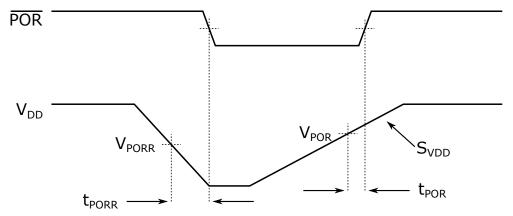
**Note:** When  $\overline{POR}$  is low, the device is held in Reset.
