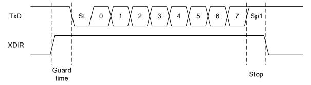
RS-485 mode is compatible with One-Wire mode. One-Wire mode enables an internal connection between the TXD pin and the USART receiver, making the TXD pin a combined TxD/RxD line.
