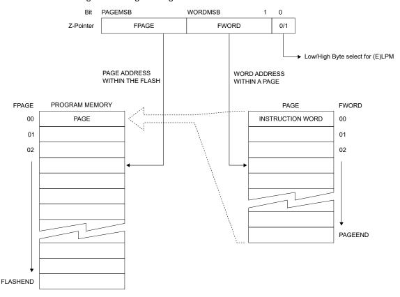
The Flash is word-accessed and organized in pages, so the Address Pointer can be treated as having two sections, as shown in the figure above. The word address in the page (FWORD) is held by the Least Significant bits (LSb) in the Address Pointer, while the Most Significant bits (MSb) in the Address Pointer hold the Flash page address (FPAGE). FWORD and FPAGE hold an absolute address to a word in the Flash.
