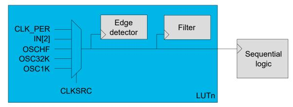
When the Clock Source (CLKSRC) bit is written to  $0 \times 1$ , LUTn-TRUTHSEL[2] is used to clock the corresponding filter and edge detector (CLK\_LUTn). The sequencer is clocked by the CLK\_LUTn of the even LUT in the pair. When CLKSRC is written to  $0 \times 1$ , LUTn-TRUTHSEL[2] is treated as OFF (low) in the TRUTH table.
