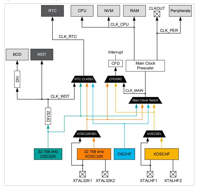
The clock system consists of the main clock and clocks derived from the main clock, as well as several asynchronous clocks:
