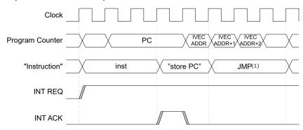
If an interrupt occurs when the device is in a sleep mode, the interrupt execution response time is increased by five clock cycles, as shown in the figure below. Also, the response time is increased by the start-up time from the selected sleep mode.
