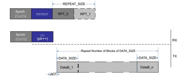
For  $\mathtt{LD}$ , data will come out continuously after the  $\mathtt{LD}$  instruction. Note the guard time on the first data block.
