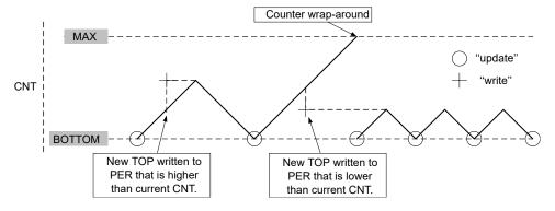
**With Buffering:** When using double-buffering, the buffer can be written at any time and still maintain the correct operation. TCAn.PER is always updated on the UPDATE condition, as shown
