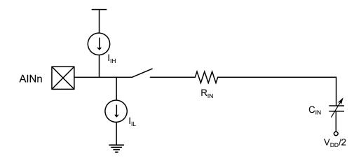
If a source with high impedance is used, the sampling time may need to be increased. The required sample time will depend on how long the source needs to charge the  $C_{\text{IN}}$  capacitor and can be configured using the Sample Duration (SAMPDUR) bit field in the Control E (ADCn.CTRLE) register.
