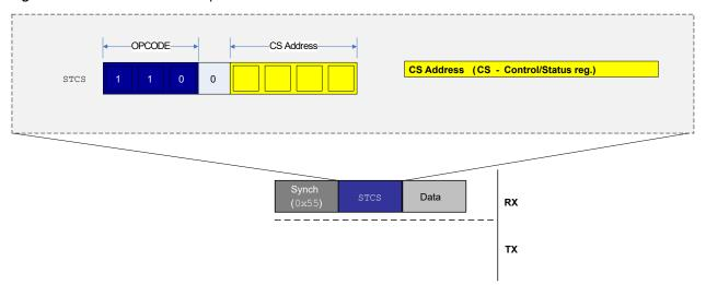
Figure 33-14 shows the data frame transmitted after the SYNCH character and the instruction frames. The STCS instruction byte can immediately be followed by the data byte. There is no response generated from the STCS instruction, as is the case for the ST and STS instructions.
