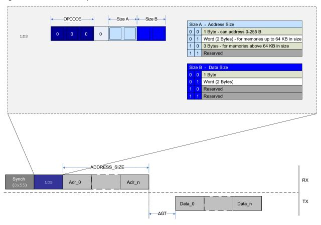
When the instruction is decoded and the address byte(s) are received as dictated by the decoded instruction, the DL layer will synchronize all required information to the ACC layer. This will handle the bus request and synchronize data buffered from the bus back to the DL layer, which will create a synchronization delay that must be taken into consideration upon receiving the data from the UPDI.
