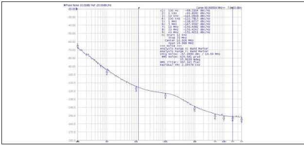
FIGURE 3-1: Typical Phase Noise @ 25°C, 100 MHz, 3.3V.
