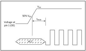
FIGURE 6-3: Enable Time with Pin 1 Configured as OE.
