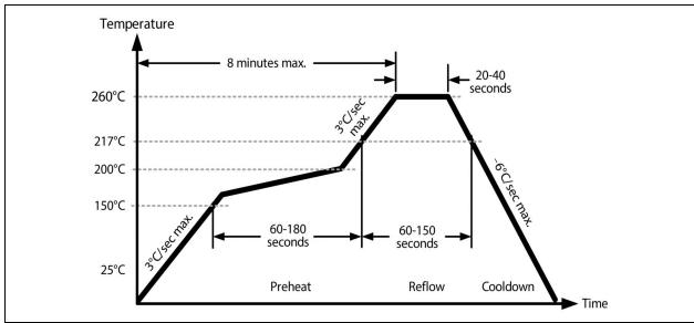
FIGURE 7-1: Solder Reflow Profile.
