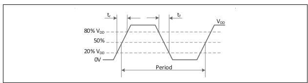
FIGURE 4-1: Output Waveform.
