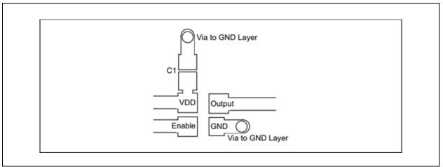
FIGURE 9-1: Recommended Board Layout.
