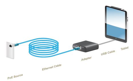
Microchip PoE to USB-C adapter connects USB-C devices to the PoE network and converts both power and data into a single USB-C connector.
