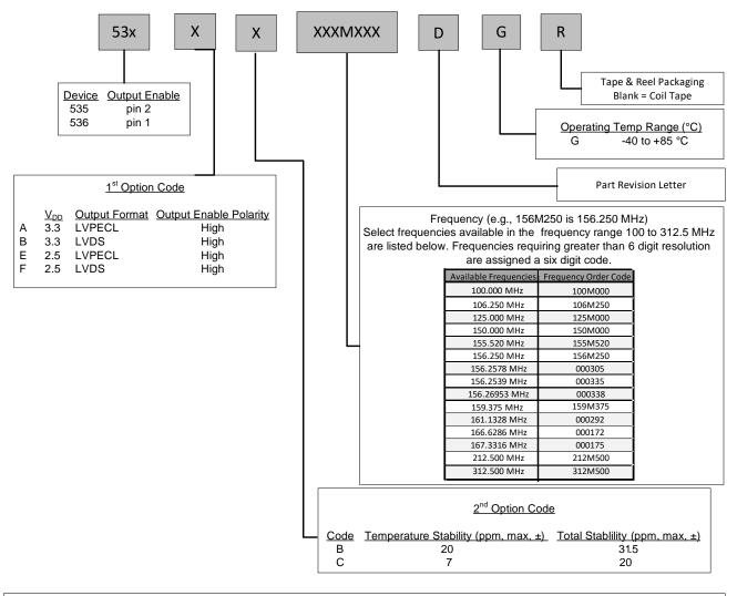
Example P/N: 535AB156M250DGR is a 5 x 7 XO in a 6 pad package. The frequency is 156.250 MHz, with a 3.3 V supply, LVPECL output, and Output Enable active high polarity. Temperature stability is specified as  $\pm 20$  ppm. The part is specified for -40 to +85 °C ambient temperature range operation and is shipped in tape and reel format.
