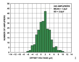
Figure 4. V<sub>OS</sub> Distribution at 25°C
