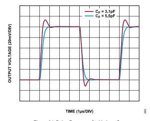
Figure 84. Pulse Response for Various C<sub>F</sub>
