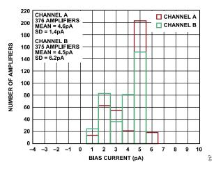
Figure 17. IB Distribution at -40°C
