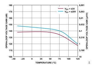
Figure 70. DC Open-Loop Gain vs. Temperature
