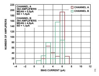
Figure 16. IB Distribution at 25°C
