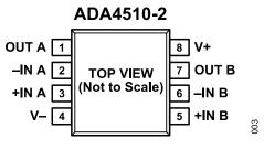
Figure 3. Pin Configuration
