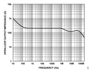
Figure 31. Z<sub>O</sub> vs. Frequency
