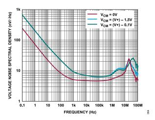
Figure 64. Input Voltage Noise Spectral Density vs. Frequency
