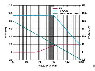
Figure 82. Compensating the TIA,  $C_F = 3.1 pF$
