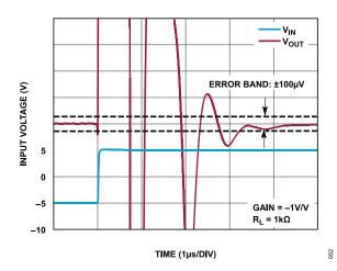
Figure 52. Positive Step Settling Time to 0.001%, V<sub>OUT</sub> = 10 V
