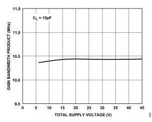
Figure 33. Gain Bandwidth Product vs. Total Supply Voltage
