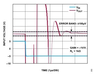
Figure 55. Negative Step Settling Time to 0.001%, V<sub>OUT</sub> = 10 V
