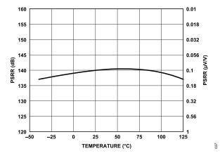
Figure 37. PSRR vs. Temperature
