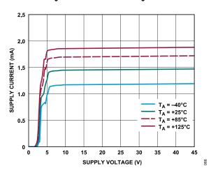
Figure 66. I<sub>S</sub> per Amplifier vs. Supply Voltage at Various Temperatures
