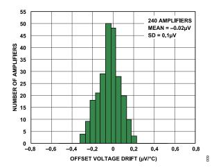
Figure 9. TCV<sub>OS</sub> Distribution from -40°C to +125°C
