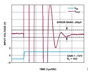
Figure 47. Positive Step Settling Time to 0.001%, V<sub>OUT</sub> = 5 V
