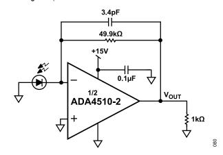
Figure 81. Single-Supply TIA Circuit Using the ADA4510-2
