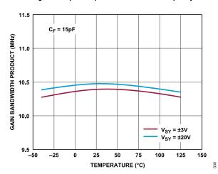
Figure 30. Gain Bandwidth Product vs. Temperature
