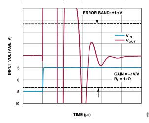
Figure 48. Positive Step Settling Time to 0.01%, V<sub>OUT</sub> = 10 V
