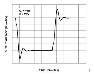
Figure 54. Small Signal Transient Response, G = 1 V/V
