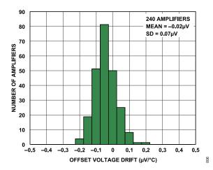
Figure 6. Input Offset Voltage Drift (TCV<sub>OS</sub>) Distribution from 0°C to +85°C
