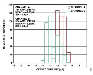
Figure 19. I<sub>OS</sub> Distribution at 25°C
