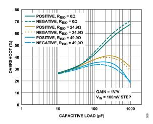
Figure 58. Overshoot vs. Capacitance Load, G = 1 V/V
