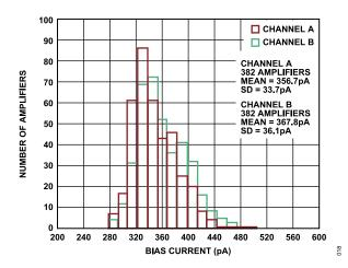
Figure 18. I<sub>B</sub> Distribution at 85°C
