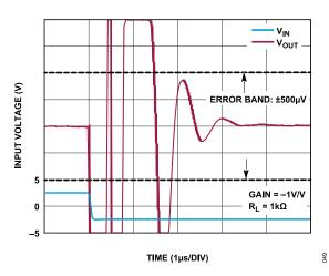
Figure 49. Negative Step Settling Time to 0.01%, V<sub>OUT</sub> = 5 V
