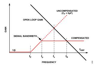
Figure 80. Generalized TIA 1/β and Transfer Function
