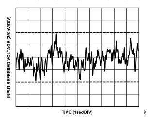
Figure 65. 0.1 Hz to 10 Hz Voltage Noise
