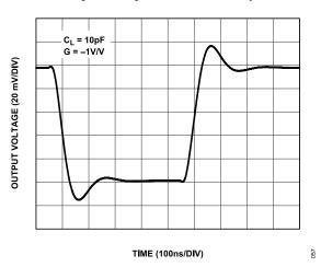
Figure 57. Small Signal Transient Response, G = −1 V/V
