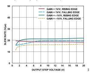
Figure 60. Slew Rate vs. Output Step Voltage
