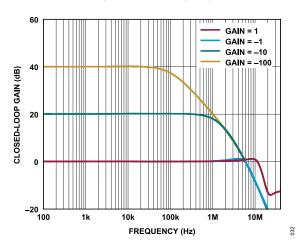
Figure 32. Closed-Loop Gain vs. Frequency
