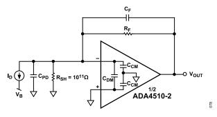
Figure 79. Equivalent TIA Circuit
