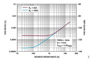
Figure 42. THD Ratio vs. Source Resistance
