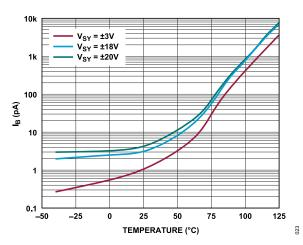
Figure 23. I<sub>B</sub> vs. Temperature
