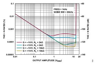
Figure 43. THD Plus Noise (THD + N) Ratio vs. Output Amplitude
