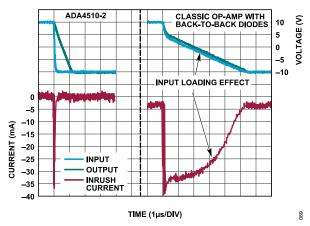
Figure 75. ADA4510-2 Inrush Current Reduction
