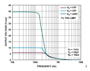
Figure 45. Maximum Undistorted Output Swing vs. Frequency
