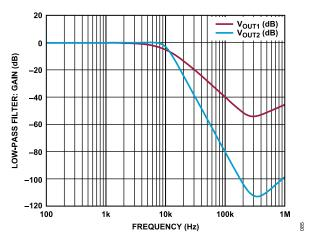
Figure 86. Low-Pass Filter: Gain vs. Frequency
