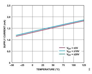
Figure 69. I<sub>S</sub> per Amplifier vs. Temperature for Various Supplies
