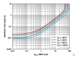
Figure 27. V<sub>DROPOUT</sub> (V<sub>OUT</sub> - (V-)) vs. I<sub>OUT</sub> Sink
