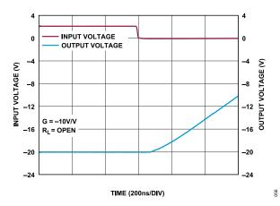
Figure 56. Negative Overload Recovery
