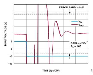
Figure 51. Negative Step Settling Time to 0.01%, V<sub>OUT</sub> = 10 V
