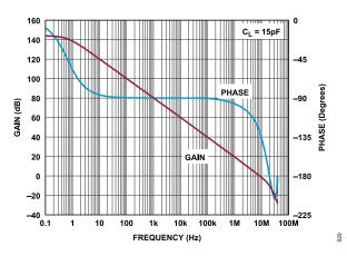
Figure 29. Open-Loop Gain and Phase vs. Frequency
