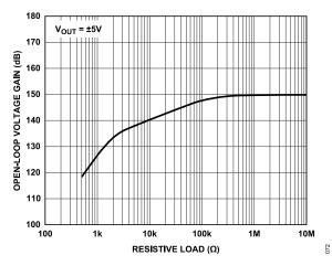
Figure 72. DC Open-Loop Gain vs. R<sub>L</sub>
