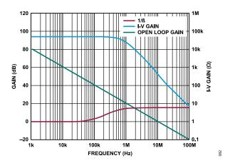
Figure 83. Compensating the TIA,  $C_F = 5.5 pF$
