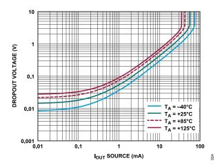
Figure 24. V<sub>DROPOUT</sub> ((V+) - V<sub>OUT</sub>) vs. I<sub>OUT</sub> Source
