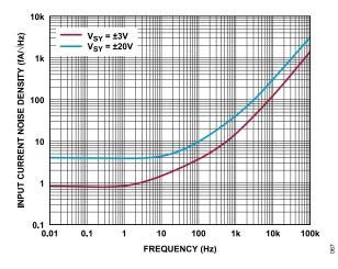
Figure 67. Current Noise Spectral Density vs. Frequency
