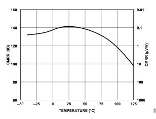
Figure 38. CMRR vs. Temperature
