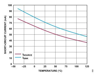
Figure 68. Short-Circuit Output Current vs. Temperature
