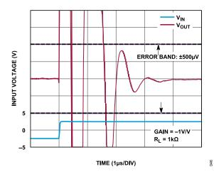
Figure 46. Positive Step Settling Time to 0.01%, V<sub>OUT</sub> = 5 V
