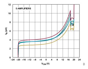
Figure 22. I<sub>B</sub> vs. V<sub>CM</sub>
