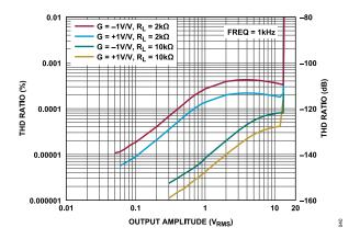
Figure 40. THD Ratio vs. Output Amplitude
