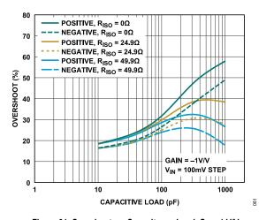
Figure 61. Overshoot vs. Capacitance Load, G = -1 V/V
