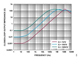
Figure 28. Z<sub>OUT</sub> vs. Frequency
