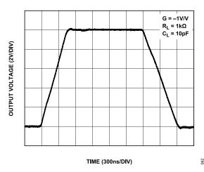
Figure 62. Large Signal Transient Response, G = -1 V/V
