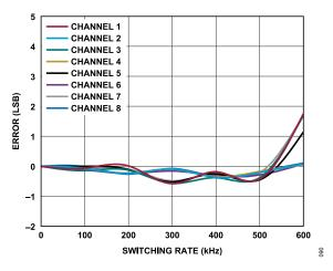
Figure 78. Error (LSB) vs. Switching Rate, 8-Channel 10 V Step
