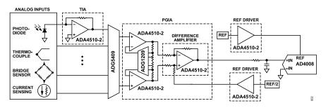
Figure 2. Multiplexed Data Acquisition Signal Chain
