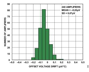
Figure 1. Ultralow Offset Voltage Drift for Precision Design
