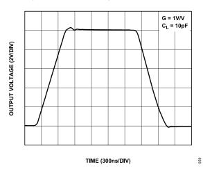
Figure 59. Large Signal Transient Response, G = 1 V/V
