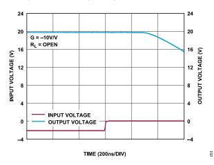
Figure 53. Positive Overload Recovery
