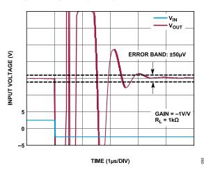
Figure 50. Negative Step Settling Time to 0.001%, V<sub>OUT</sub> = 5 V
