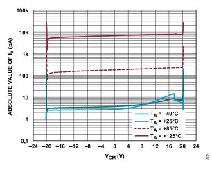
Figure 25. I<sub>B</sub> vs. V<sub>CM</sub>, Four Temperatures
