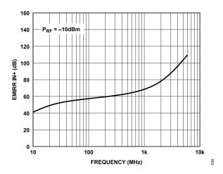
Figure 36. EMIRR IN+ vs. Frequency (P<sub>RF</sub> Is RF Power.)
