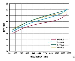
Figure 16. NPR vs. Frequency over Current, 73 dBmV TCP, 18 dB Tilt
