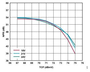
Figure 10. NPR vs. TCP over Voltage, 1041 MHz, 20 dB Tilt
