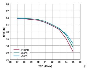
Figure 8. NPR vs. TCP over Temperature, 1041 MHz, 20 dB Tilt
