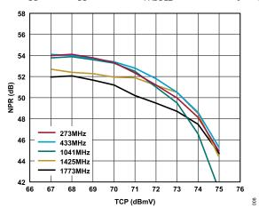
Figure 7. NPR vs. TCP over Frequency, 20 dB Tilt
