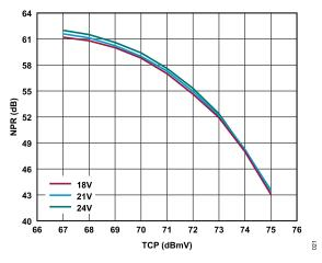
Figure 20. NPR vs. TCP over Voltage, 111 MHz, 13 dB Tilt
