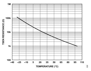
Figure 27. TSEN Resistance vs. Temperature
