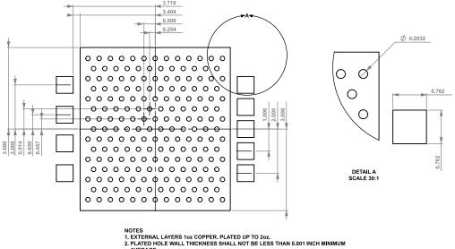
AVERAGE. 3. THRU VIAS FILLED WITH NON-CONDUCTIVE EPOXY AND PLATED OVER. DRILL 0.2032mm FINISHED HOLES AT 0.254mm.
