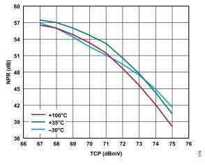
Figure 15. NPR vs. TCP over Temperature, 111 MHz, 18 dB Tilt
