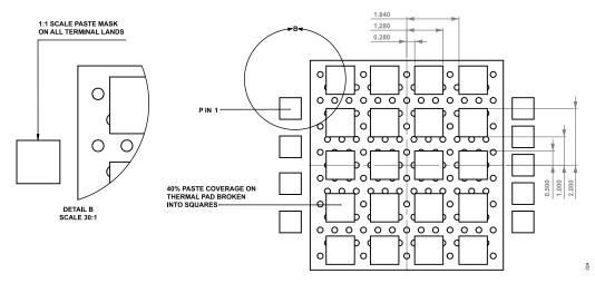
Figure 23. Recommended Solder Pattern (Dimensions Shown in Millimeters)
