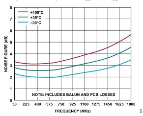
Figure 21. Noise Figure vs. Frequency over Temperature
