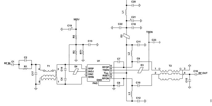
Figure 24. Recommended Application Circuit Schematic
