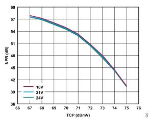
Figure 17. NPR vs. TCP over Voltage, 111 MHz, 18 dB Tilt
