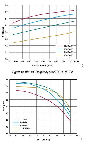
Figure 14. NPR vs. TCP over Frequency, 13 dB Tilt
