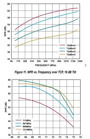
тср (dBmV) Figure 12. NPR vs. TCP over Frequency, 18 dB Tilt
