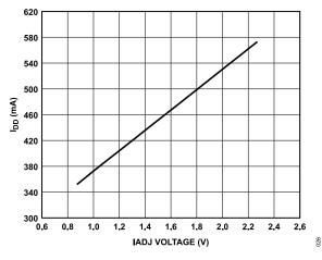
Figure 25. I<sub>DD</sub> vs. IADJ Voltage over V<sub>DD</sub>
