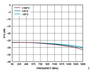
Figure 4. S12 vs. Frequency Over Temperature
