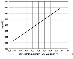
Figure 26. IDD vs. Application Circuit IADJ Voltage over VDD
