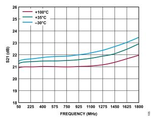
Figure 5. S21 vs. Frequency Over Temperature
