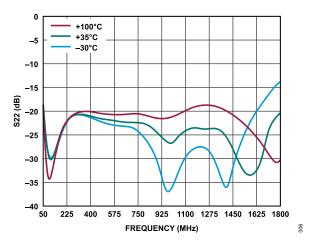
Figure 6. S22 vs. Frequency Over Temperature
