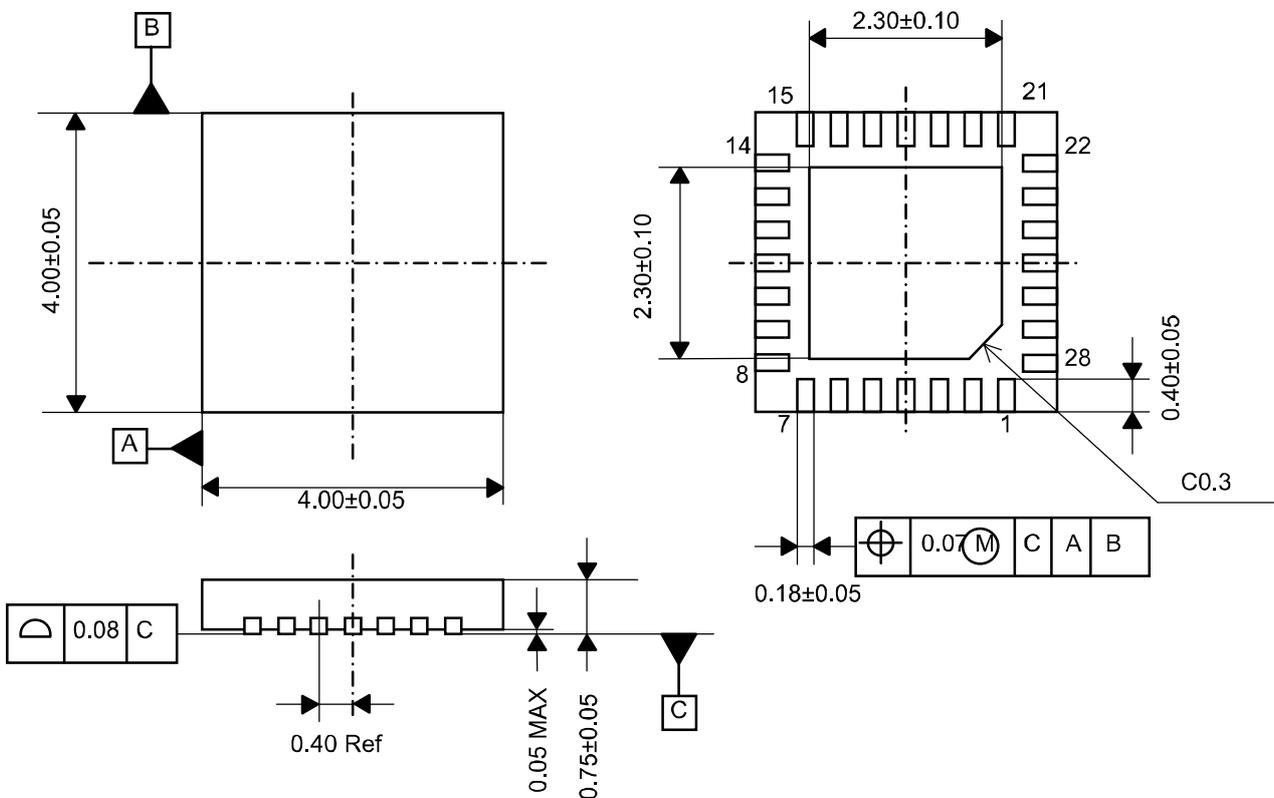
Note) The exposure pad(Exposed Pad) of the center of the package back is connected to opening or VSS.
