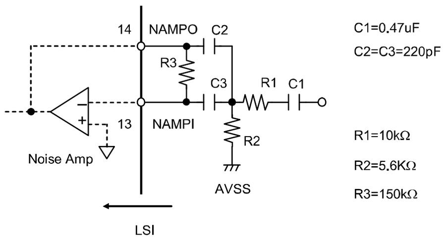
$$(1) f_0 = \frac{1}{2\pi\sqrt{R_3(R_1 // R_2)C^2}}$$
