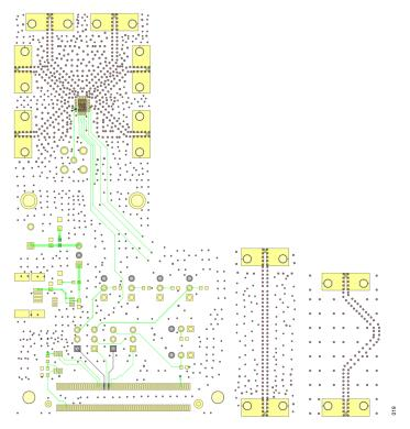
Figure 19. EVAL-ADGM1121SDZ Component Side PCB Drawing (Layer 1)
