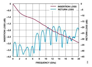
Figure 9. Calibration Transmission Line Insertion Loss and Return Loss
