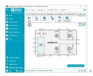
Figure 5. EVAL-ADGM1121SDZ Block Diagram with Labels
