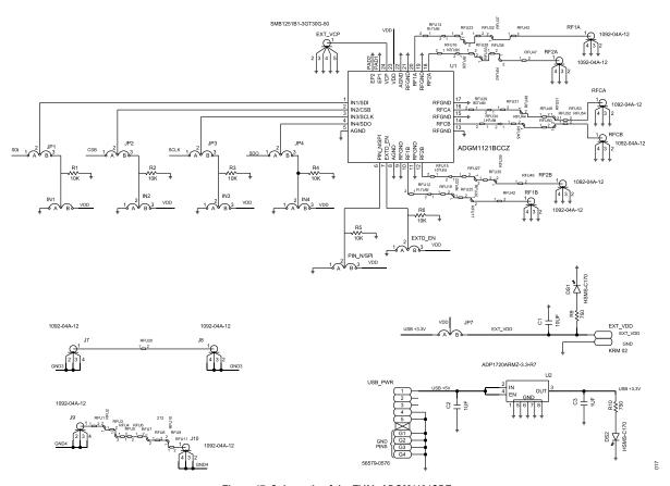
Figure 17. Schematic of the EVAL-ADGM1121SDZ
