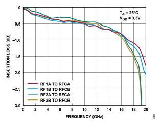
Figure 11. PCB De-Embedded ADGM1121 Insertion Loss Performance
