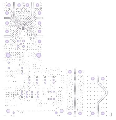
Figure 20. EVAL- ADGM1121SDZ Component Side Ground Plane PCB Drawing (Layer 2)
