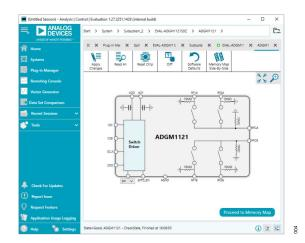
Figure 4. Chip Block Diagram View for the ADGM1121
