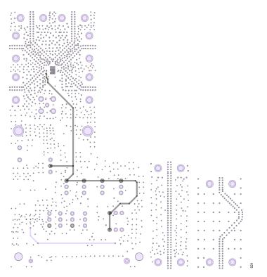
Figure 21. EVAL- ADGM1121SDZ Component Side Ground Plane PCB Drawing (Layer 3)
