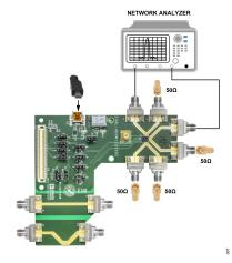
Figure 7. EVAL-ADGM1121SDZ Connection Diagram for Parallel-Interface
