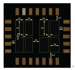
Figure 16. Solder Stencil Recommendations in Millimeters
