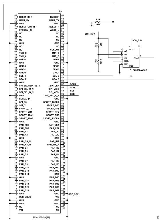
Figure 18. Schematic of the EVAL-ADGM1121SDZ with an SDP Connector
