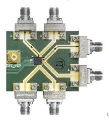
Figure 10. Calibration Transmission Line Length Equal to the A + B Length
