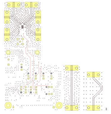
Figure 22. EVAL- ADGM1121SDZ Component Side, Bottom Side PCB Drawing (Layer 4)
