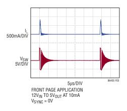
Figure 3. Burst Mode Operation
