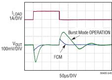
FRONT PAGE APPLICATION 100mA TO 1.1A TRANSIENT  $12V_{IN}$ ,  $5V_{OUT}$ ,  $f_{SW}=1MHz$   $C_{OUT}=100\mu F$
