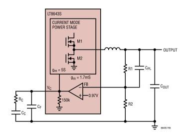
Figure 5. Model for Loop Response
