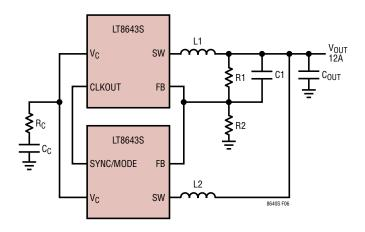
Figure 6. Paralleling Two LT8643Ss
