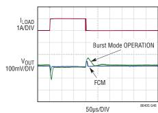
$C_{C}$  = 330pF,  $R_{C}$  = 6.49k,  $C_{LEAD}$  = 4.7pF 100mA TO 1.1A TRANSIENT 12V<sub>IN</sub>, 5V<sub>OUT</sub>, f<sub>SW</sub> = 1MHz  $C_{OUT}$  = 100µF
