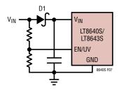
Figure 7. Reverse V<sub>IN</sub> Protection
