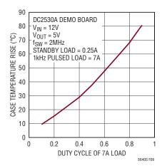
Figure 9. Case Temperature Rise vs 7A Pulsed Load
