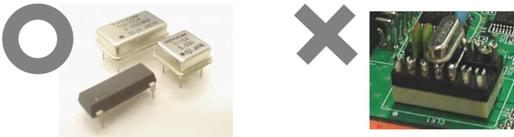
Figure 2-2. Oscillator Shape
