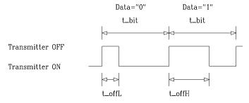
Figure 5-6. Write Pulse Timing for TXCT-
