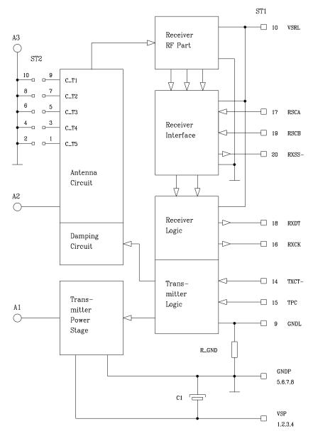
Figure 2-1. Mini-RFM Block Diagram
