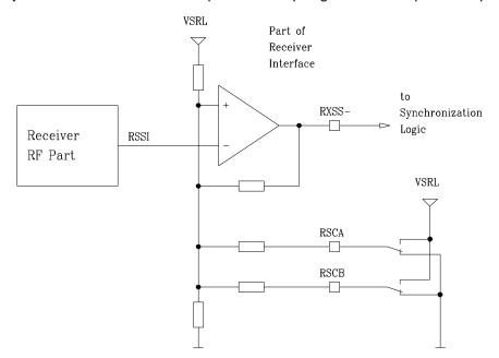
Figure 5-4. Synchronization Output Control - Digital Adjustment
