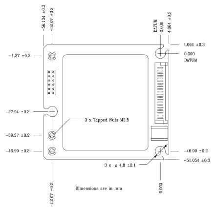
Figure 4-2. Mechanical Dimensions - Top View
