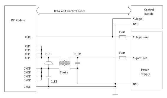
Figure 5-3. Supply Line Wiring for a Separated Power Supply
