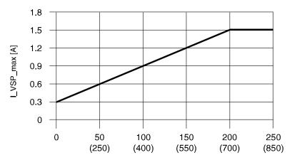
Time t\_off between 2 charge pulses of 50 ms [ms]
