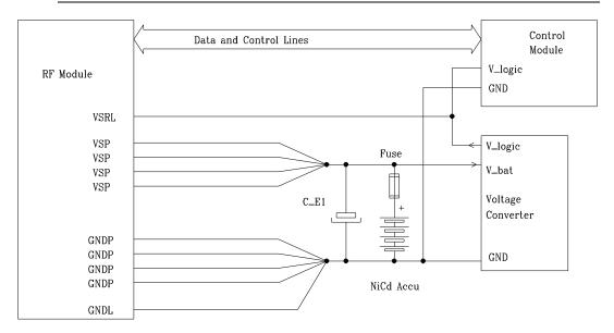
Figure 5-2. Supply Line Wiring for Short Supply Lines
