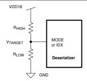
Figure 7-2. Strap Pin Connection Diagram
