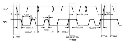
Figure 6-4. I2C Serial Control Bus Timing
