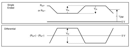
Figure 6-2. V<sup>3</sup>Link Receiver VID, VIN , VCM
