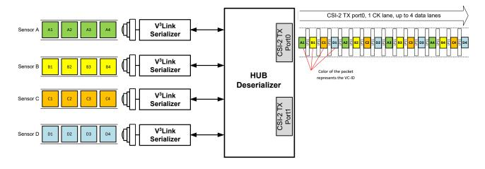
Figure 7-12. Four Sensor Data onto CSI-2 With Virtual Channels (VC-ID)
