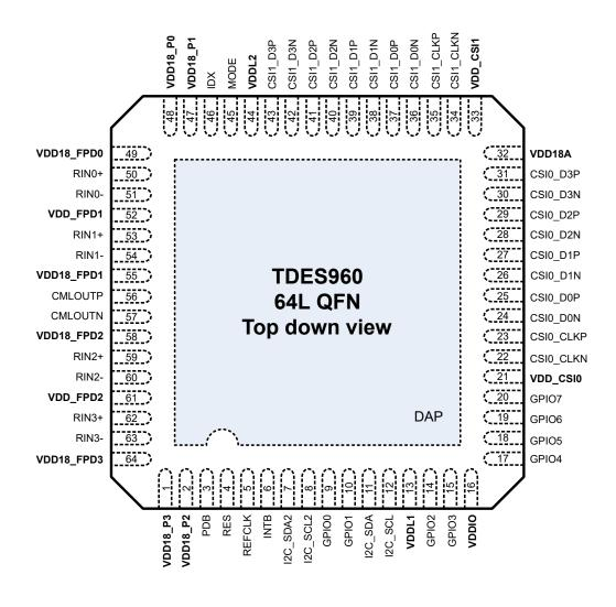
Figure 5-1. RTD Package 64-Pin VQFN (Top View)
