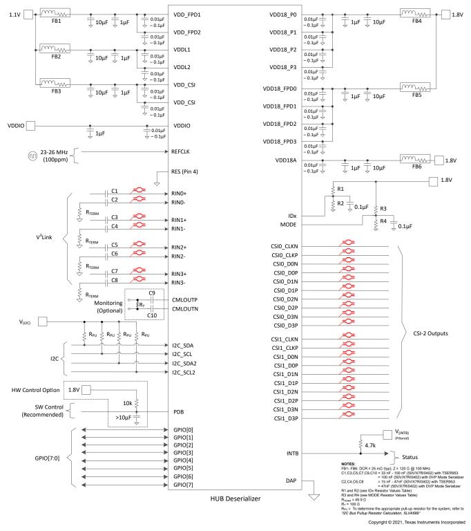
Figure 8-4. Typical Connection Diagram (Coaxial)
