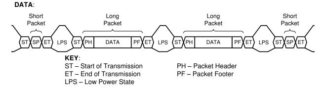
Figure 7-6. CSI-2 Protocol Layer With Short and Long Packets
