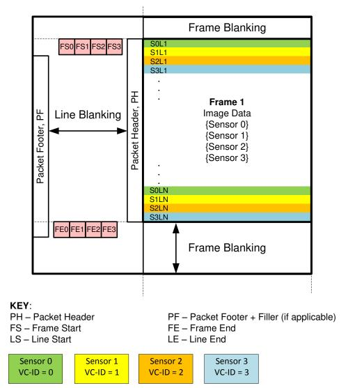
\*Blanking intervals do not provide accurate synchronization timing
