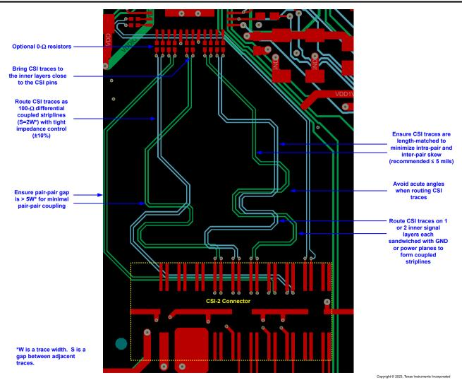
Figure 8-23. Example Routing of CSI-2 Traces
