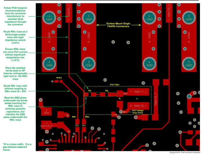
Figure 8-22. Example Routing of V<sup>3</sup>Link Traces to a Single Mini-Fakra Connector and PoC Components
