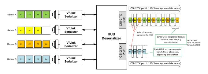
Figure 7-13. Four Sensor Data onto CSI-2 With Virtual Channels (VC-ID) With Different Frame Size
