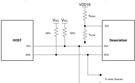
Figure 7-21. Serial Control Bus Connection
