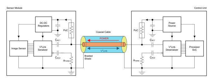
Figure 8-1. Power-over-Coax (PoC) System Diagram
