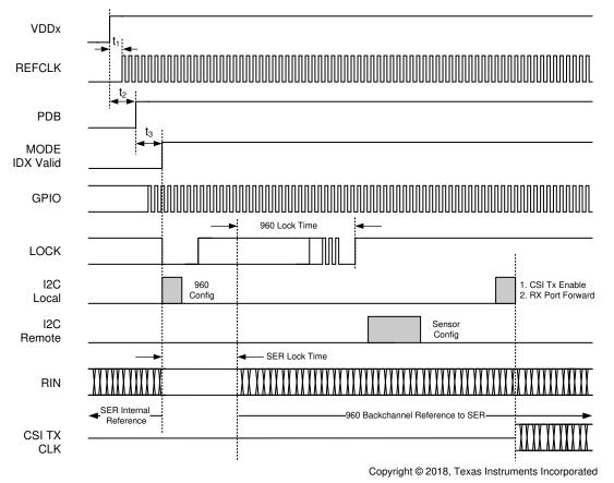
Figure 8-19. Power-Up Sequencing With Synchronous Clocking Mode
